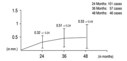
**Fig. 2.** Average subsidence in millimeters (+/-SD) after total hip replacement with lateral flare prosthesis
