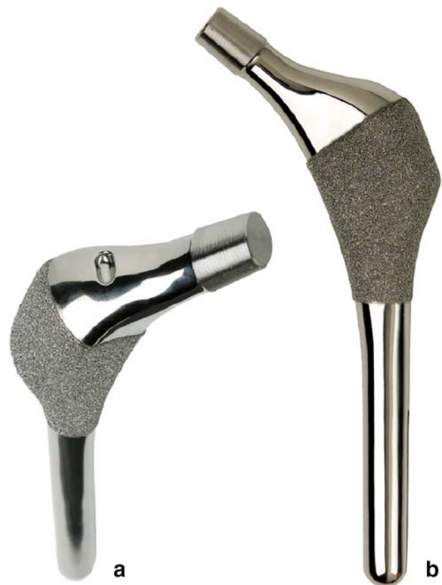
Fig. 1 a The Revelation hip stem. Top-to-bottom view of the prosthesis: the anteverted neck and the plug-type trapezoidal proximal geometry can be appreciated. b The lateral flare designed to engage the proximal lateral cortex is the distinctive feature, along with a tapered, polished distal portion to minimize distal contact
